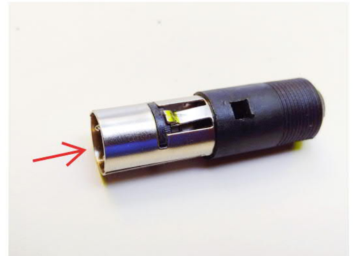
Reassemble the connector, push connector nose upwards again if needed
