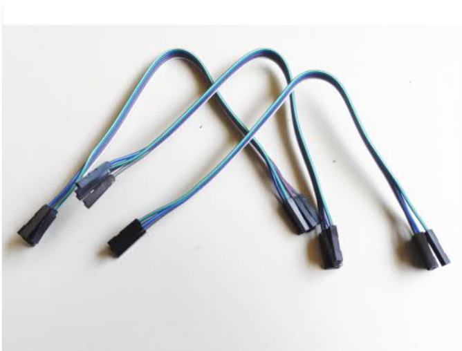
Find female to female header wires Tear off three sections with 5x identical colours
