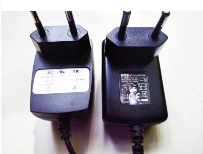
The 5V power variant can be powered by any old phone charger that delivers atleast 400mA. Also using USB cables or powerbanks is possible Do not power the 9V variant from 5V - it may behave erratically
