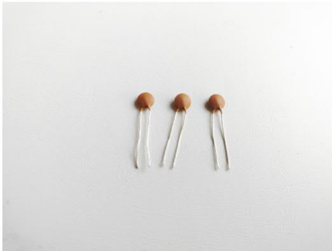
Find 3x capacitor 0.1uF Body marking 104
