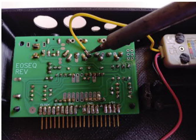
Solder yellow wire to shown pin on midi out
