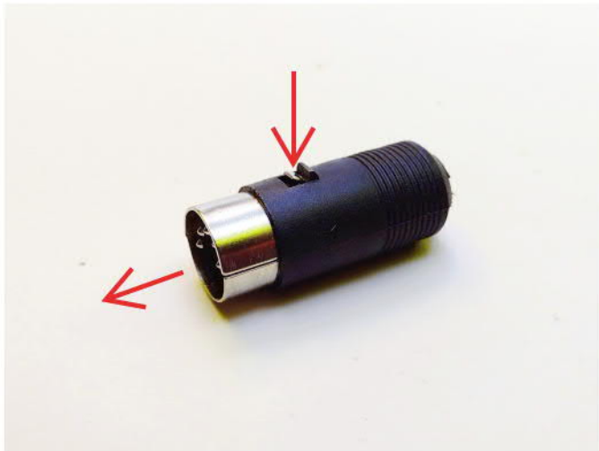
Internal soundcard Midi Out loopback adapter Find 5 PIN DIN connector, push connector nose and disassemble
