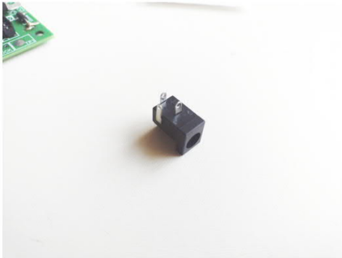
Find PSU socket Alternate part might have different pins and shielding
