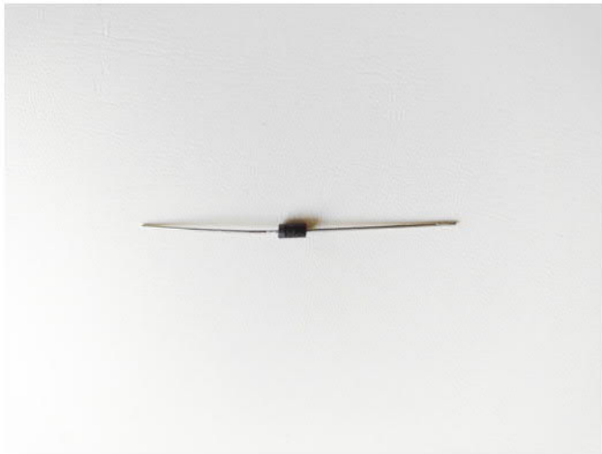
Find diode 1N4004 Black body colour Alternate part: 1N4001
