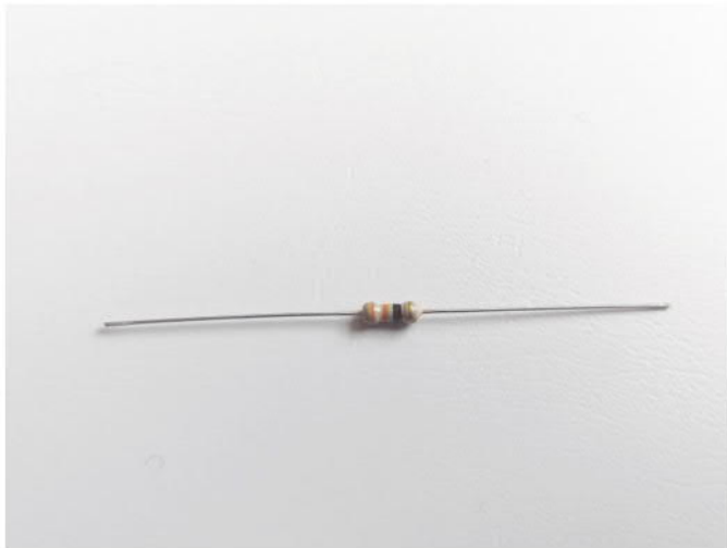
Find resistor 33 Ohm Orange Orange Black Gold
