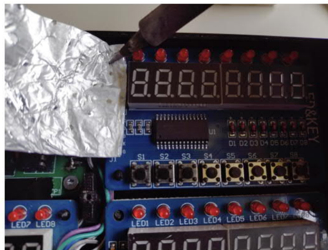
Optional for stability: Melt down all TM1638 mounting pins with aluminium foil, normally the three TM1638 pcb's will stay in their place when the top plate is mounted
