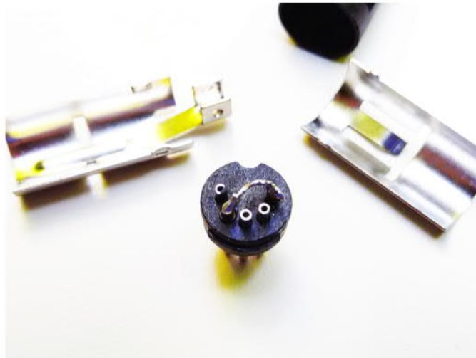
Use a clipped off component leg or piece of wire to install the bridge as shown This routes midi output from Eosequencer back to midi input of the M5 SAM2695 synth, using a pin that is commonly unused for midi connections.
