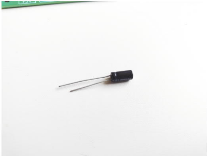
Find capacitor 4.7\mu\text{F} \geq 50\text{V}
