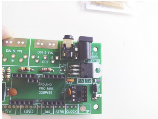
Put PSU socket into place
