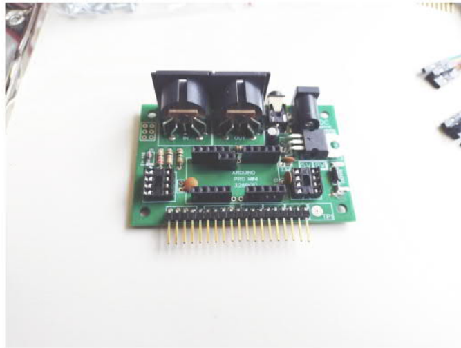
Put 90° pins into place
