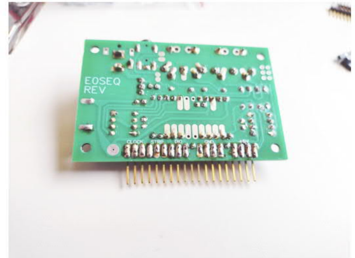
Solder 90° pins in place
