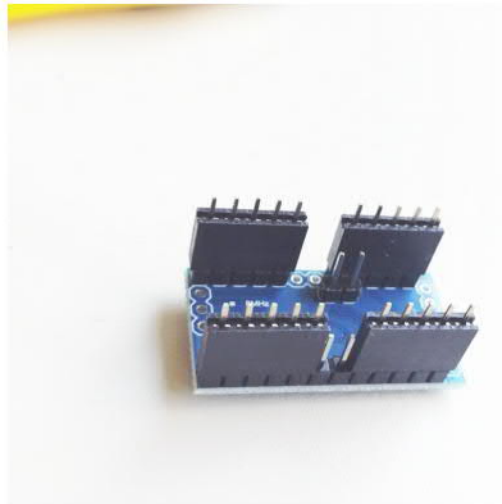
Mount 4x 5pin header sockets as shown
