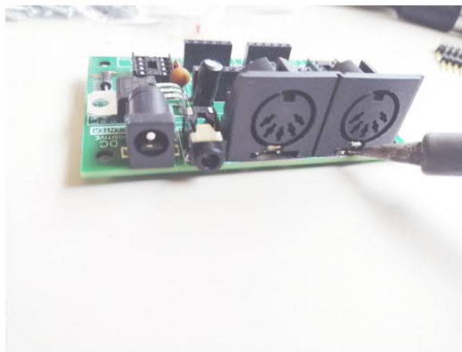
Optional for more stability: Solder grounding tab to pcb
