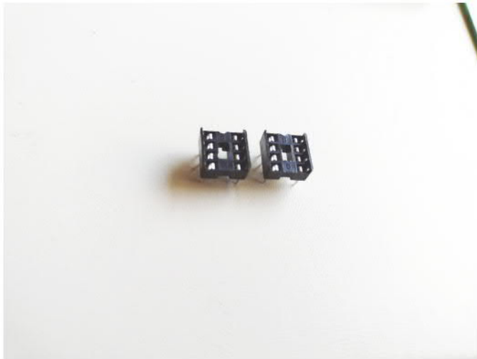
Find 2x 8 pin IC sockets
