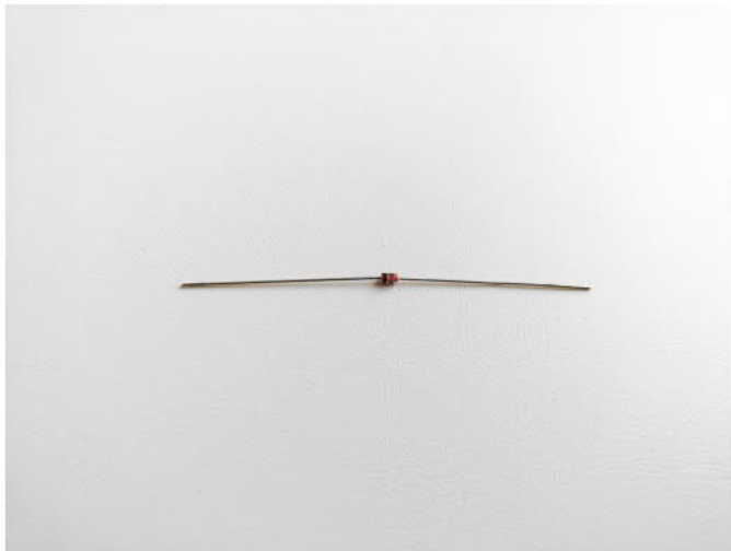
Find diode 1N4531 Red body colour Alternate part: 1N4148
