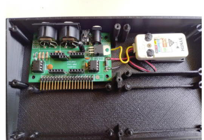
Route wires as shown M5 SAM2695 installation done
