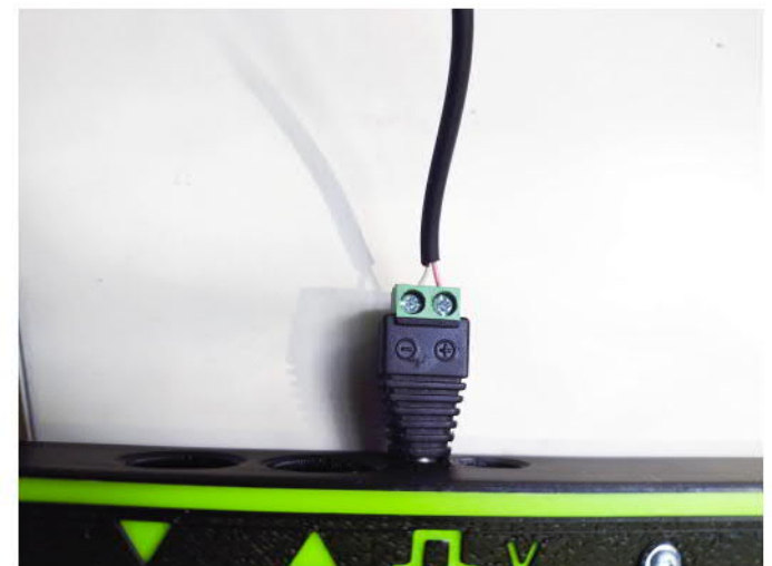
Since the pcb has a polarity protection diode, just attach the wires and check if it powers up. If not, swap the wire On a USB power / data cable use only the red and black wires, insulate other wires (white, green etc.)
